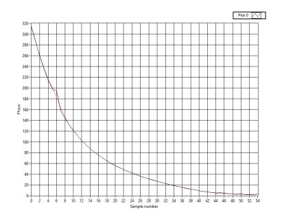
3). The fitting curve with image number based on its name is converted to the voltage (in V), which is out final plot. Also by using the "Interpolate 1D" to fit this plot to find the voltage (in V) corresponds to the phase of 90°, with a phase retardance accuracy of 0.1°. Save this array data in you code by using "Data Operation"  $\rightarrow$  "Make Current Data Default"  $\rightarrow$  then save you code
